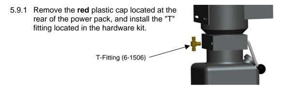
5.9.2 Bolt power pack to the mounting bracket on the power side tower using hardware from the kit. **Do not tighten.**
