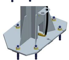
If anchor bolts do not tighten to 150 ft-lbs. OR project more than 1 ¾" above the concrete surface, the concrete MUST be replaced by an appropriate concrete pad. (Consult Product Manufacturer / Supplier for further details).
