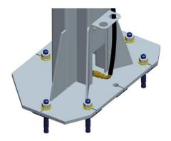
If anchor bolts do not tighten to 150 ft-lbs. OR project more than 1 ¾" above the concrete surface, the concrete MUST be replaced by an appropriate concrete pad. (Consult Product Manufacturer / Supplier for further details).
