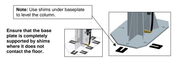
**WARNING!** Do not use more than  $\frac{1}{2}$ " (13mm) of shims. Anchor bolts supplied allow for a maximum of  $\frac{1}{2}$ " (13mm) of shim. If more than  $\frac{1}{2}$ " (13mm) of shims are required, DO NOT proceed with installation and contact Product Manufacturer / Supplier for further details.
