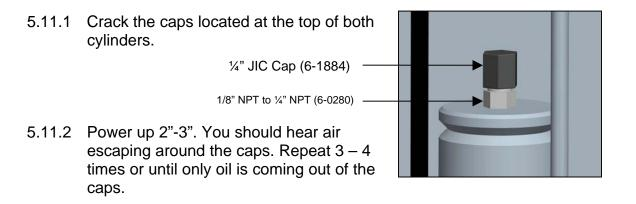
5.11.3 Tighten the caps and lower the lift.
