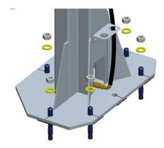
Check that the column is level front to rear and side to side. Adjust shims as required.
