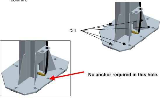
5.12.4 Clean out the drilling dust from the holes and hammer in the anchor bolts. **Hand tighten all anchor bolts.**
