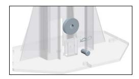
5.5.6 Route equalizing cable around pulley and reassemble the pulley to the base plate.
