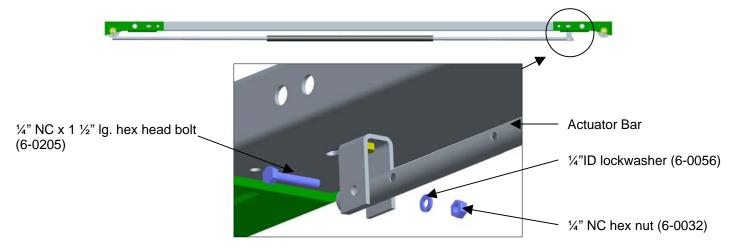
5.4.3 Slide Safety Shut-Off Microswitch Assembly over the open end of actuator bar.
