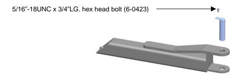
5.6.2 Install the four arms on the carriages by inserting the arm pins.
