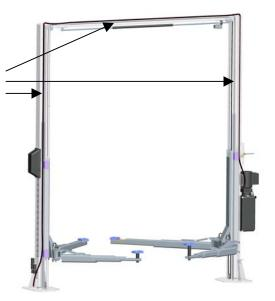
5.10.5 Remove the plastic cap from the bottom of the slave side cylinder and connect the long hose to the cylinder.
