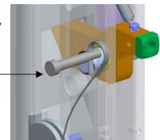
Pull cable out through the opening in tower and route under large pulley.
