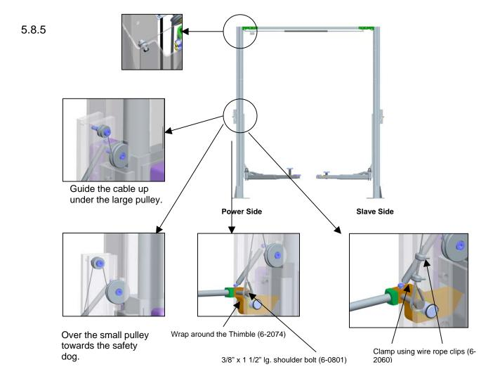
Do not tighten fully at this stage.
